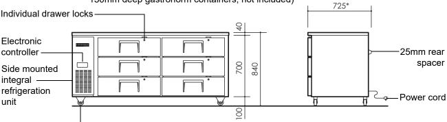
Swivel castors (front locking) or four adjustable legs (100-160mm)
